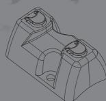
Support for 1 and 2 mm wires. Use: To make angles from 90° to 170° - for angles bigger than 90° should be used 2 pieces.
