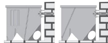
With the new hopper's guides, it is possible to use also the wax blocks. To use this tool, break the hopper's central arc; then insert the hopper in the vertical guides and the block in the featured rod. You may place the rod inside the station in vertical or horizontal position. Meal bait, pellets or seed can be used with the hopper in the usual guides.
