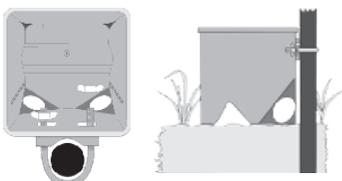
The included "U" hook allows fixing Ristorat to rounded poles or other vertical standings with cm 2,5 - 6 diametres. To lock the Ristorat to the pole use the wing nuts.
